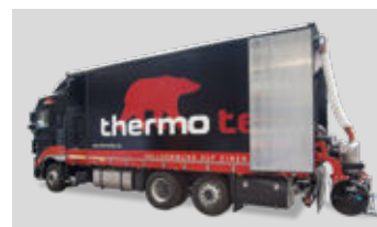
Delivery, mixing and pumping are carried out by the thermotec® Mixmobiles
